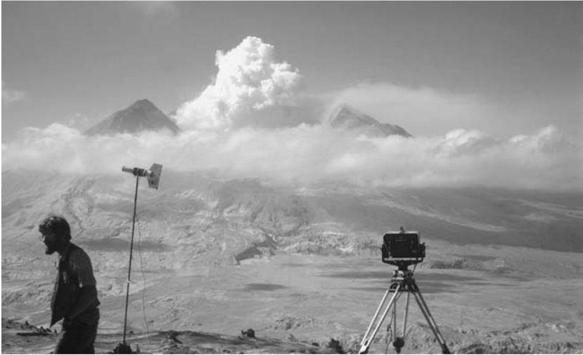
Laser survey instrument setup north of Mount Saint Helens, August 6, 1980. This is a highly accurate technology that enables the user to measure changes on the slope from a safe distance. [M. Lukk and the U.S. Geological Service]
