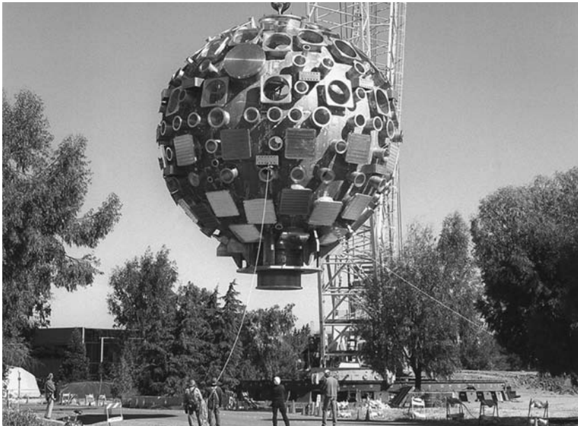
This is the target chamber of the National Ignition Facility, a 1-million-pound, 10-meter-diameter aluminum sphere that functions as the interface between a target, high-energy lasers, and numerous measurement devices. The laser system can produce a pulse equal in power to 1,000 times the electric generating power of the United States. [U.S. Department of Energy]
