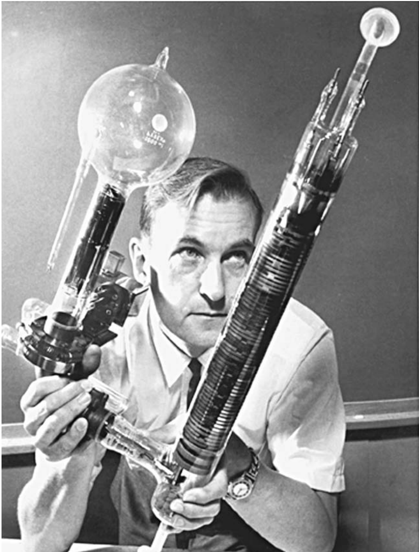
This laser emits its beam in the ultraviolet. It was one of the first commercially available lasers to emit its energy in that part of the electromagnetic spectrum. [Mary Evans Picture Library/The Image Works]
