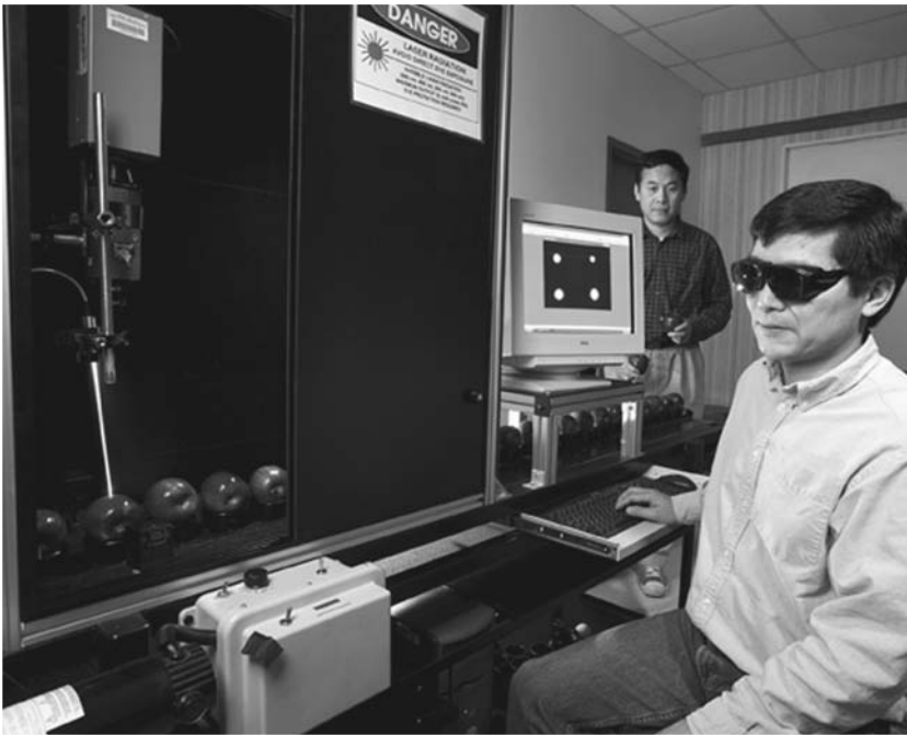
Spectroscopy is now a highly developed science. Spectrometers come in a variety of designs and have found application in many different fields. In this photo, a prototype laser-based spectrometer called a multispectral imaging system is used to measure the firmness and sugar content of apples. [Stephan Rusmus and U.S. Department of Agriculture]
